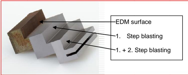
By that used in the first stage of the  $\mu$ -kro-blasting method abrasive blasting agents this martensite is removed to 100%. This works in seconds and most importantly without
