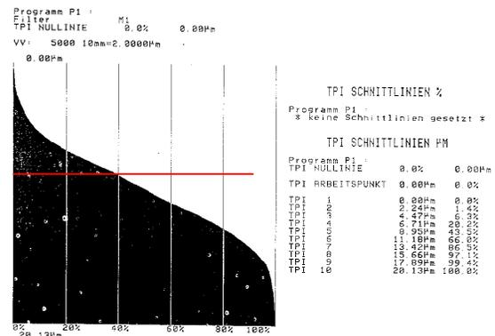
After the µ-kro-blasting treatment, the surface is at 40% viable after 3 microns for disposal
