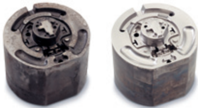
Cleaning of a zinc die-cast mould with subsequent surface compaction to reduce mould release problems
