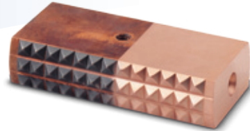
Cleaning of an electrode to extend the operating life, to inspect for surface damage and to improve the spark process
